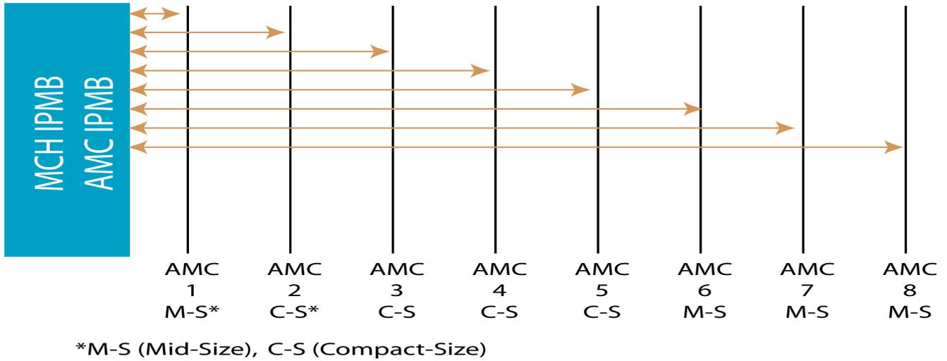
FIGURE 1. VT875 Topology for AMC I2C Bus
