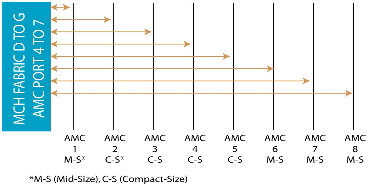
FIGURE 5. VT875 Topology for AMC Ports 4-7
