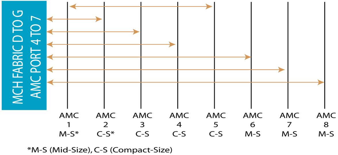
FIGURE 4. VT875 Topology for AMC Ports 4-7 with direct connect across two slots
