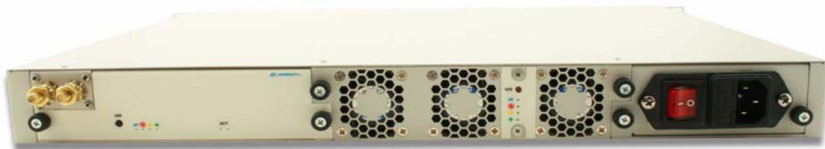
Rear view with AC and DC power supply option
